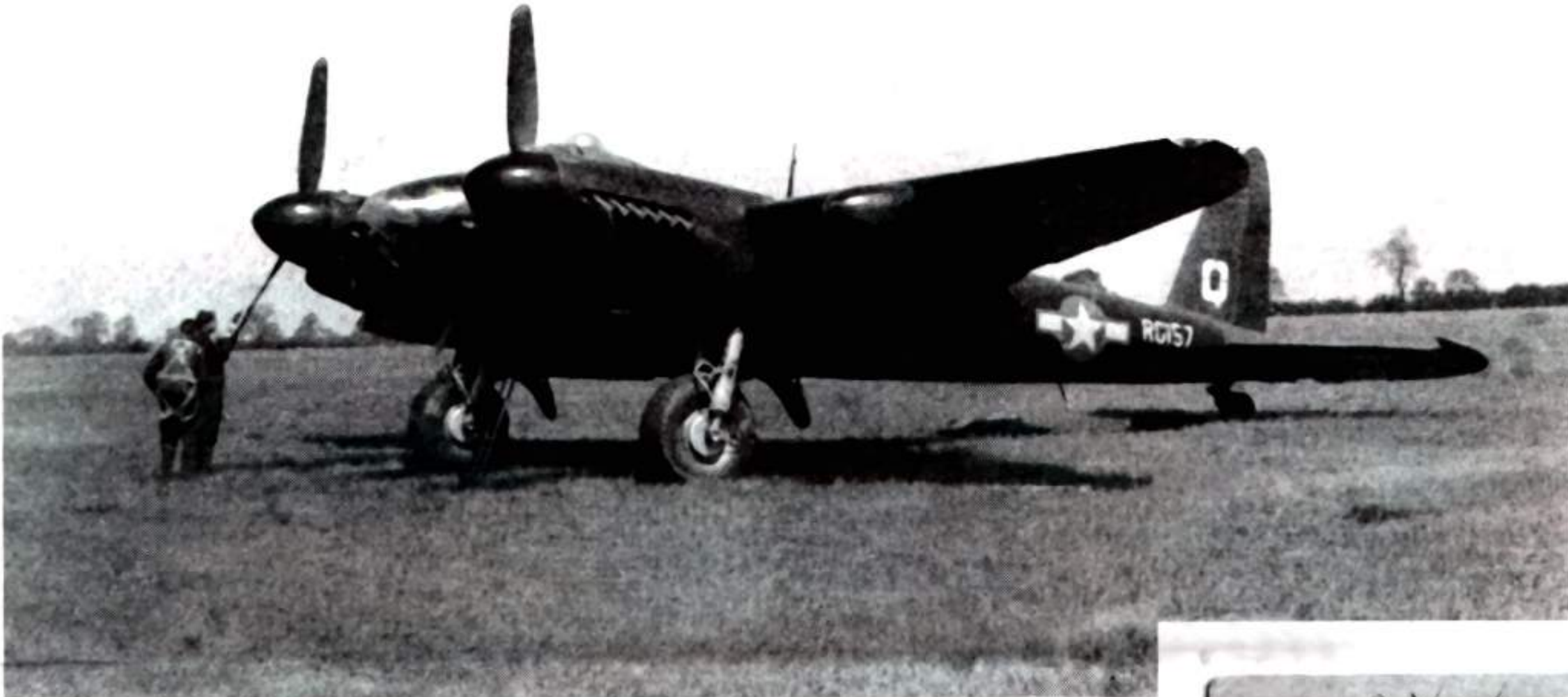
Our deHavilland Mosquito spy plane could climb to 40,000 feet at a speed of more than 400 miles per hour: not bad for an airplane made primarily of wood. The British-made, propeller-driven aircraft was affectionately known as the "Mossie." It was painted a gloss-black and was powered by two Rolls Royce Merlin engines.
